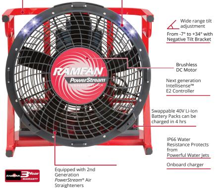
Note: Output changes as setback from the opening changes. Single door airflow is per AMCA 240-15 testing, This data derives from 0" static pressure. Real world results will be substantially reduced by structure backpressure. EX50Li is tested at at 12.7° tilt and 2924 rpm on AC Power Supply and tested at 14 ft (4.3 m) setback at 9° tilt and 3045 rpm on DC Power Supply.
